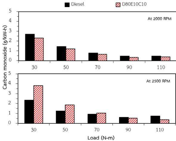
Figure 7. Carbon monoxide emissions
