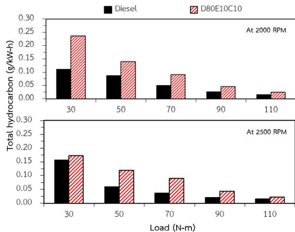
Figure 6. Unburnt hydrocarbon emissions
