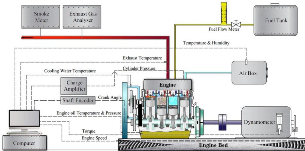
Figure 1. Schematic diagram of the experimental installation
