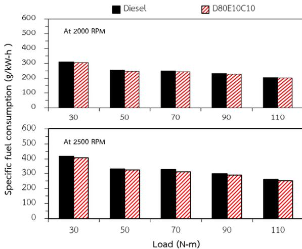
Figure 2. Brake specific fuel consumption
