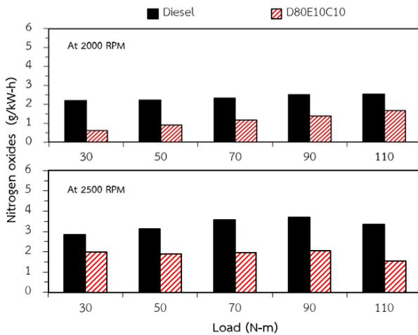
Figure 8. Nitrogen oxide emissions
