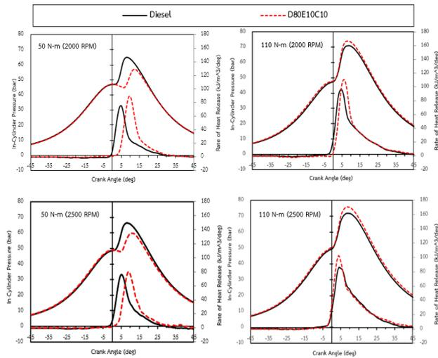
Figure 4. In-cylinder pressure and heat release rate
