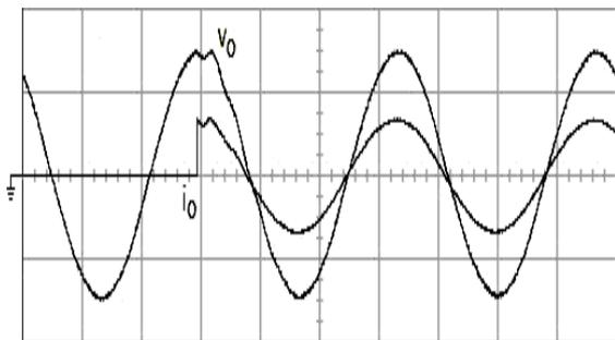
Figure 2. Proposed control technology with sudden load change (100V/div; 20A/div; 5ms/div).
