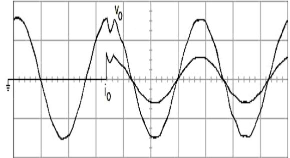
Figure 3. Traditional SMC with sudden load change (100V/div; 20A/div; 5ms/div).
