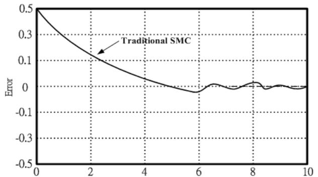
Figure 5. Tracking error convergence rate with traditional SMC.
