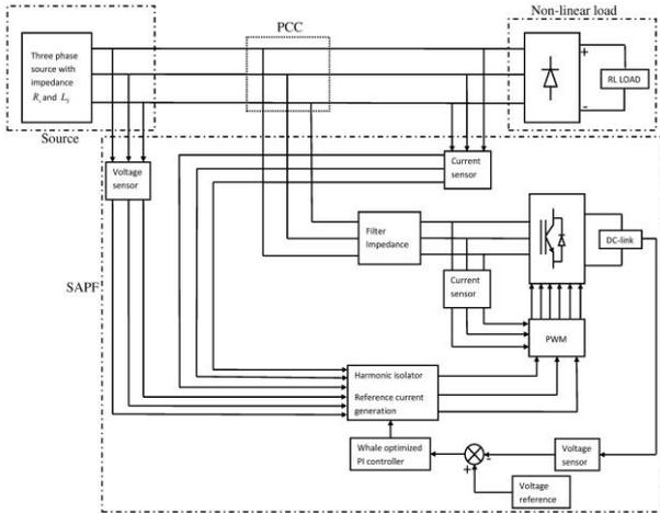
Figure 1. Block diagram of SAPF
