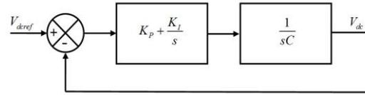
Figure 4. Voltage control loop
