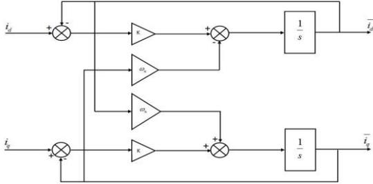
Figure 3. Block diagram of STF
