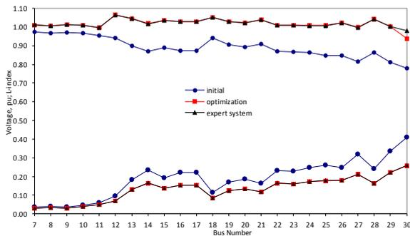
Figure 2. Voltage and L-index profile of modified IEEE-30 Bus system.
