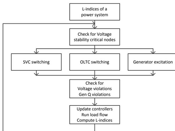
Figure 1. Proposed expert system for voltage stability improvement.
