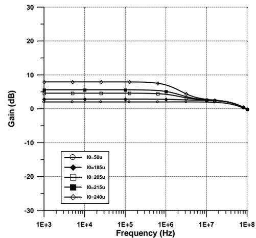
Figure 10. Inverting all-pass filter's electronically tunable gain response.
