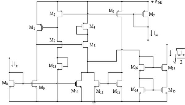
Figure 1. Current-mode square-root-domain circuit.
