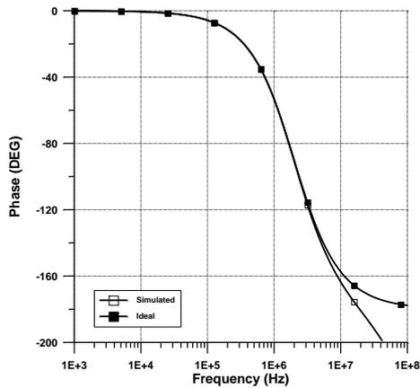
Figure 7. Inverting all-pass filter's phase response.
