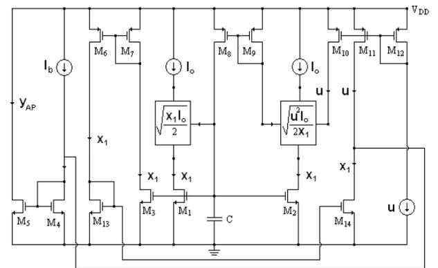
Figure 5. Square-root-domain current-mode first order non-inverting all-pass filter circuit.
