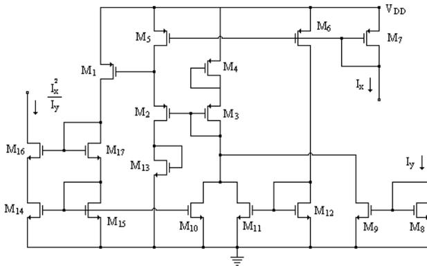
Figure 2. Current-mode squarer/divider circuit.
