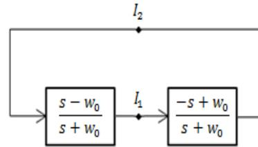
Figure 14. Block diagram for quadrature oscillator.
