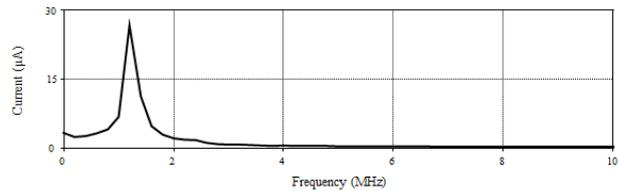
Figure 17. The output spectrum of the oscillator.
