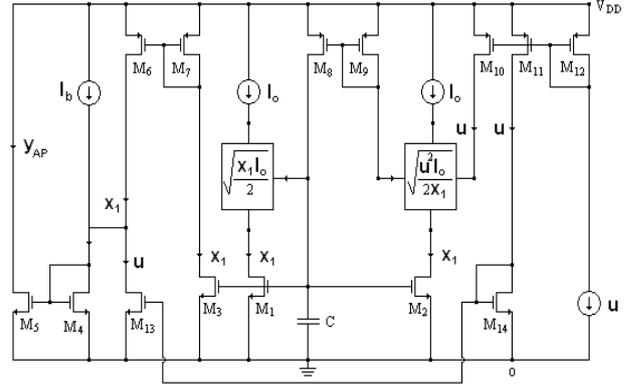
Figure 4. Square-root-domain current-mode first order inverting all-pass filter circuit.
