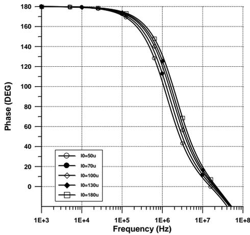
Figure 13. Non-inverting-all-pass filter's electronically tunable phase response.
