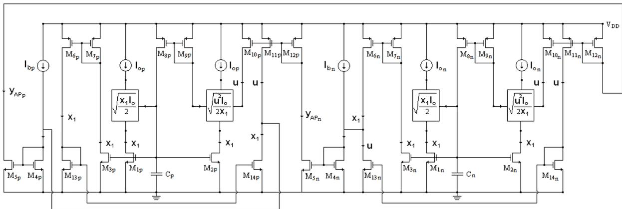
Figure 15. Square-root-domain quadrature oscillator.
