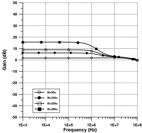
Figure 12. Non-inverting all-pass filter's electronically tunable gain response.
