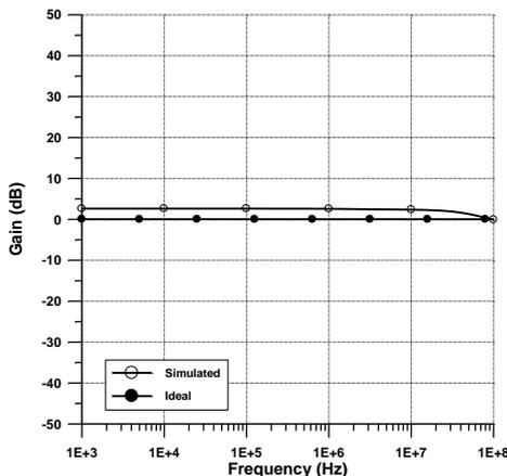
Figure 8. Non-inverting all-pass filter's gain response.
