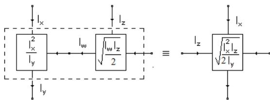
Figure 3. Sub-circuit 2: Current-mode square-root circuit connected to squarer/divider circuit Current-mode square-root circuit.
