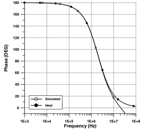
Figure 9. Non-inverting all-pass filter's phase response.
