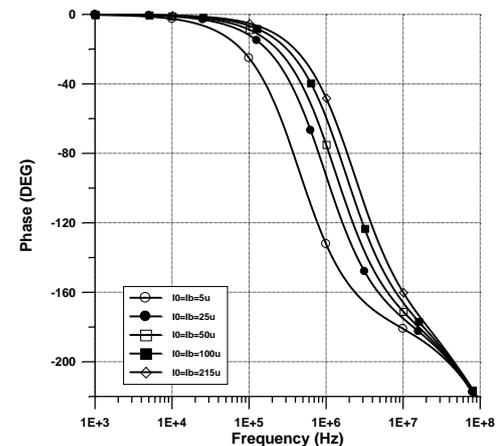
Figure 11. Inverting all-pass filter's electronically tunable phase response.
