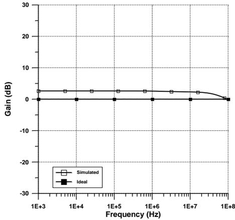
Figure 6. Inverting all-pass filter's gain response.
