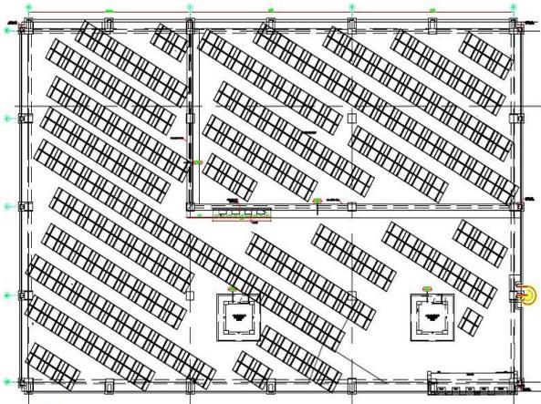
Figure 9. Lay out of PV system (top view)
