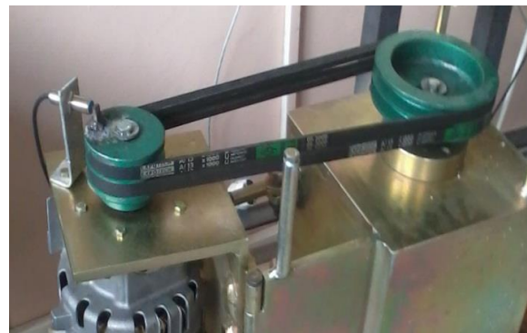
Figure 4. Measurement system of asynchronous generator speed.
