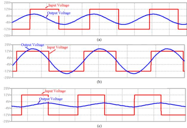
Figure 7. Voltage waveforms as output vs. input for LCR circuit at frequencies: (a) 975kHz, (b) 1.066MHz and (c) 1.4MHz.
