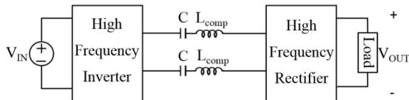
Figure 3. Conventional capacitive WPT system architecture [1].
