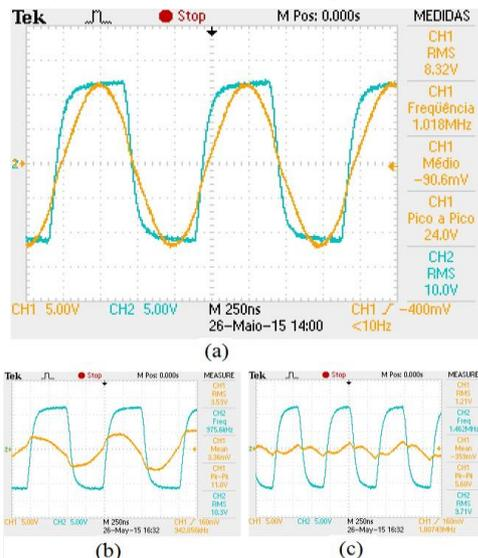
Figure 9. Voltage waveforms as output vs. input for LCR prototype at frequencies: (a) 1.018MHz, (b) 975kHz and (c) 1.4MHz.
