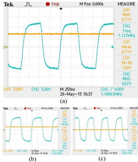
Figure 10. Voltage waveforms as output vs. input for LCR prototype at frequencies: (a) 1.137MHz, (b) 996kHz and (c) 1.4MHz.
