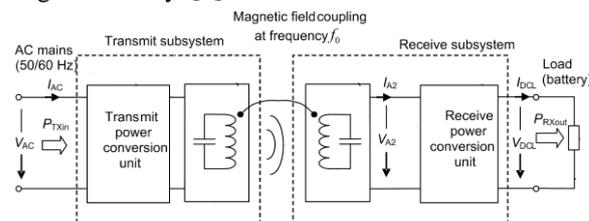
Figure 1. Wireless inductive power transfer example [9].
