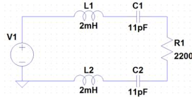
Figure 6. LCR circuit simulated to verify resonating frequency.
