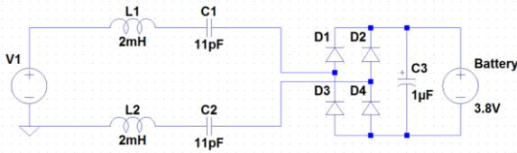
Figure 5. Main circuit structure proposed for a low power mobile device charging application.
