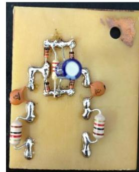
Figure 11. Prototype LCR circuit with Load resistor, rectifier and C filter.
