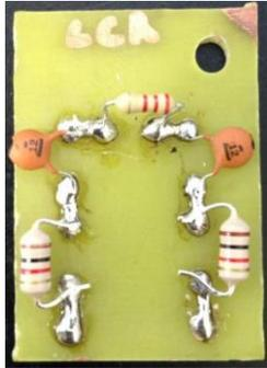
Figure 8. Prototype LCR circuit with load resistor.
