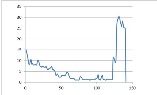
Figure 4. Leakage current in a 24 hour period.
