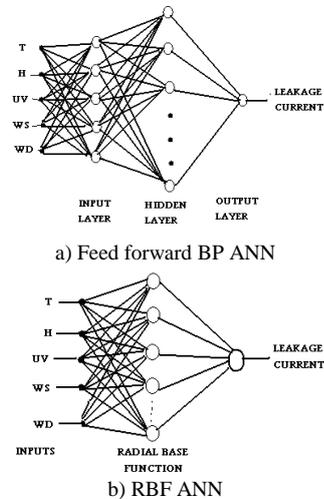
Figure 5. BP and RBF neural networks schematics.
