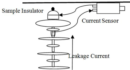
Figure 3. An LC sensor-insulator connection.
