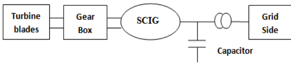
Figure 1. Wind turbine system with SCIG [1]
