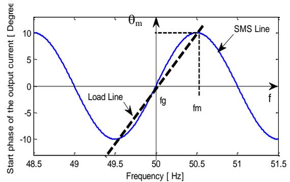
Figure 4. SMS sinusoidal frequency shift.
