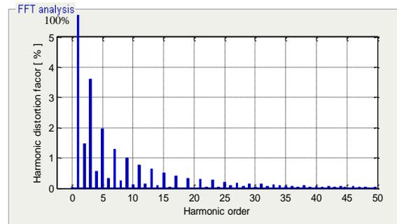
Figure 7. Harmonic spectra of inverter output currents with AFD method.
