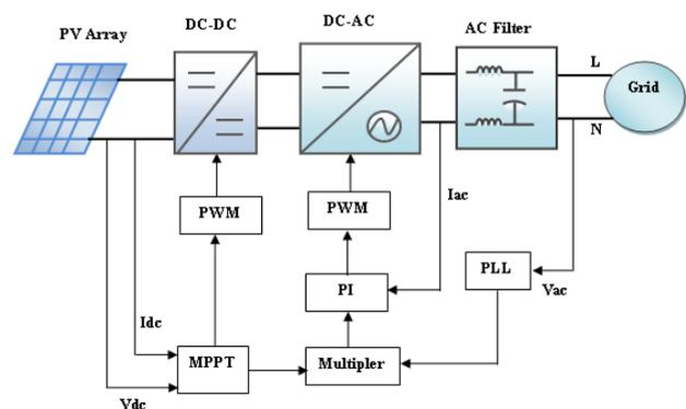
Figure 1. A block diagram of a PV system using single phase grid PV inverter with a current control.
