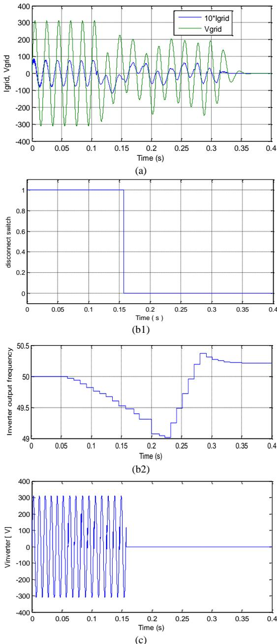
Figure 5. Islanding test results at around zero grid power flow condition: SMS method.
