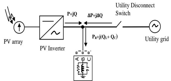
Figure 3. PV inverter test circuit for islanding.
