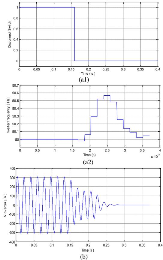
Figure 6. Islanding test results at around zero grid power flow condition: AFD method.
