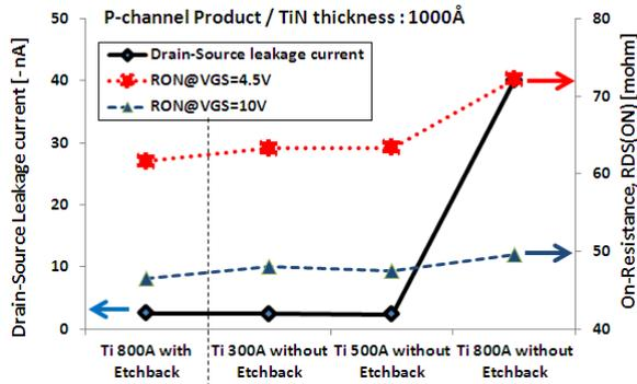
Figure 4. Drain-source leakage current and ON resistance for various Ti thickness and with or without Ti/TiN etchback
