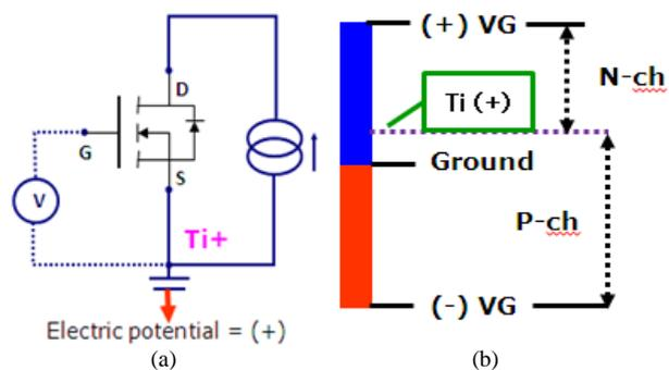
Figure 7. (a) Equivalent circuit for Threshold voltage test. (b) Electrical potential between Gate and Source.
