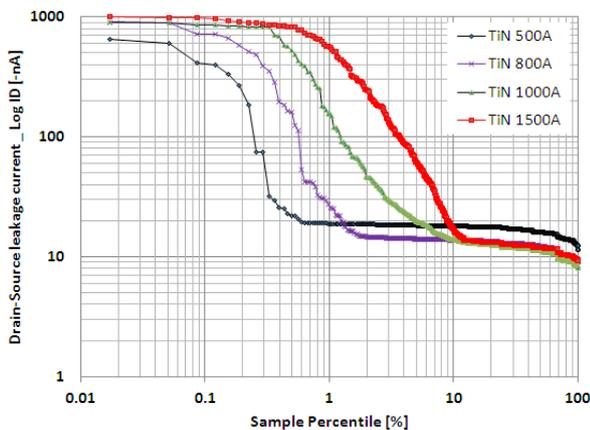
Figure 8. Probability chart of drain-source leakage current for various TiN thickness.
