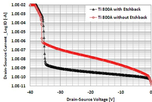
Figure 2. VD-ID graph regarding the Ti/TiN etchback effect for P-channel -30V device.
