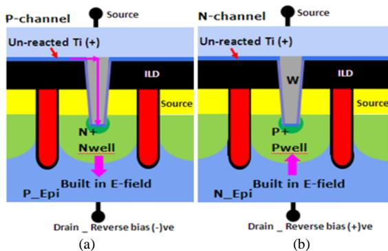
Figure 5. The direction of built in electrical field in (a) N-channel device (b) P-channel device, illustrating for leakage current increase only P-channel device due to un-reacted Ti (+) ion.
