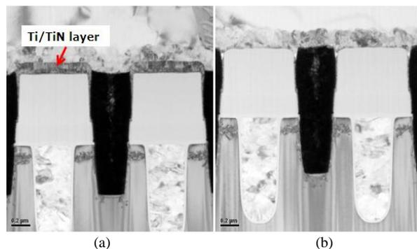
Figure 3. TEM cross sectional picture for (a) remain Ti/TiN layer on top of ILD (b) all removed Ti/TiN layer.
