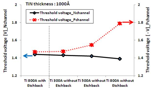
Figure 6. Threshold voltage for various Ti thickness and with or without Ti/TiN etchback
