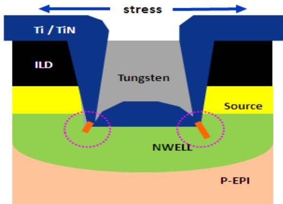
Figure 9. Zoom out cross sectional of Trench contact structure after barrier metal formation.
